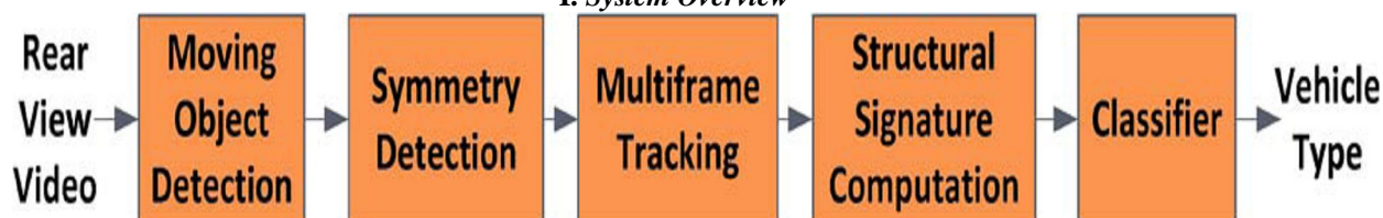
Fig. 2 System for vehicle classification.[1]
