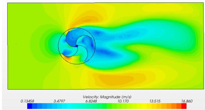
Fig.8: Velocity profile of VAWT
