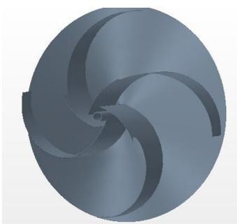
Fig.9 VAWT with gap between shaft and blades
