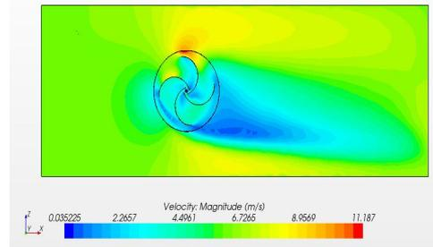
Fig.12: Velocity profile of VAW
