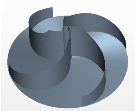
Fig.5: VAWT with no gap between shaft and blades.
