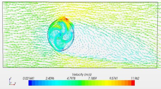
Fig.11: Velocity profile of VAWT
