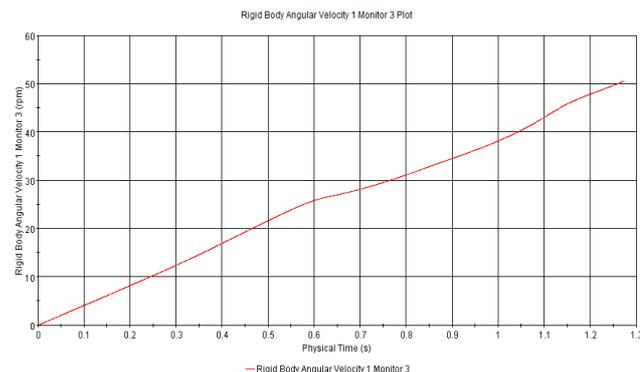
Fig.14 Rotation of VAWT with gap between shaft and blade
