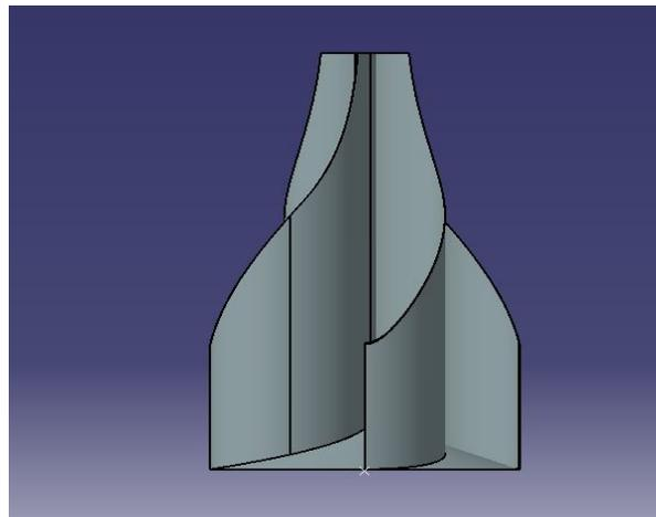
Fig.4 Vertical axis wind turbine
