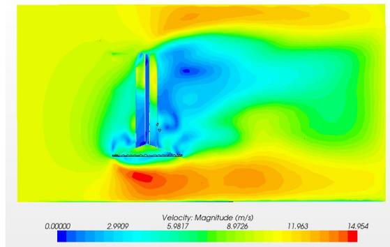
Fig.6: VAWT with wind flow.
