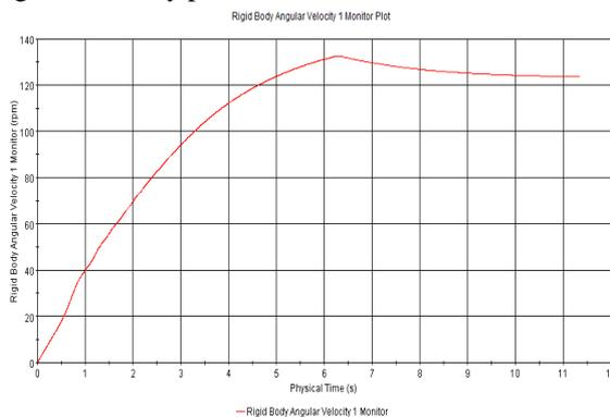
Fig.13 Rotation of VAWT without gap between shaft and blade
