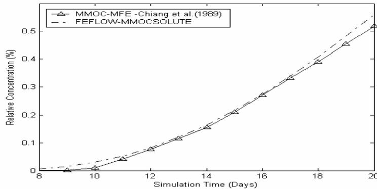
Figure 2 Comparison of concentration breakthrough curves obtained by FEFLOW-MMOC SOLUTE
