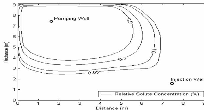
Figure 4 Solute concentration distributions by FEFLOW-MMOC SOLUTE model under the combined injection and pumping well conditions for Test Case
