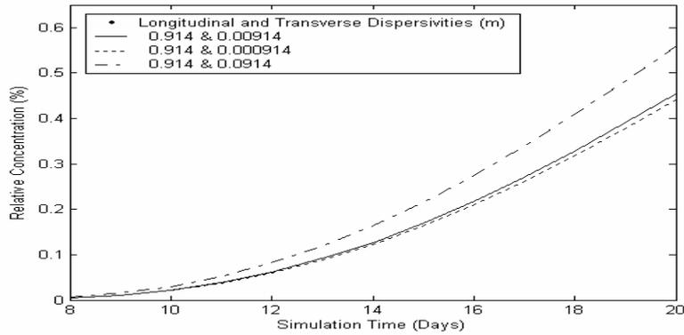
**Figure 5** Effect of dispersivity on FEFLOW-MMOCSOLUTE model solutions under the combined injection and pumping well conditions for Test Case
