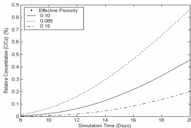
**Figure 6** Effect of porosity on FEFLOW-MMOCSOLUTE model solutions under the combined injection and pumping well conditions for Test Case
