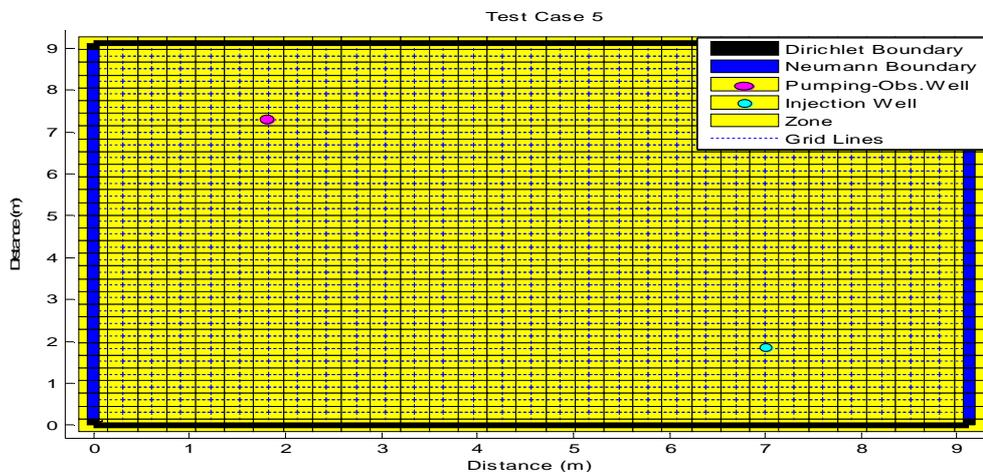
Figure 1 Schematic of aquifer modeled in Test Case for the simulation of solute transport in two-dimensional transient groundwater flow in unconfined aquifer under the combined injection and pumping well conditions
