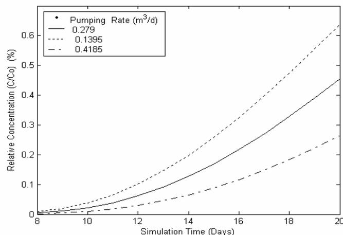
**Figure 7** Effect of combined injection and pumping rate on FEFLOW-MMOC SOLUTE model solutions for Test Case
