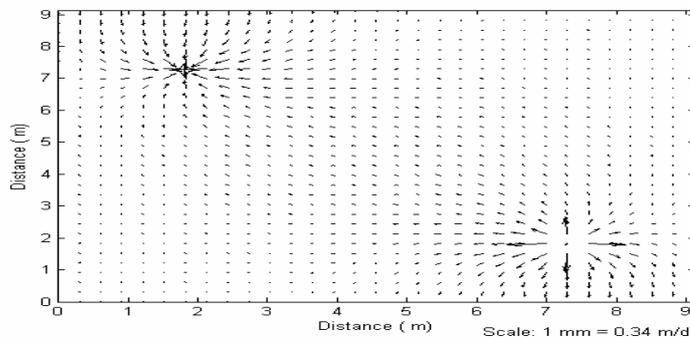
Figure 3 Simulated velocity field by FEFLOW model under the combined injection and pumping well system for Test Case
