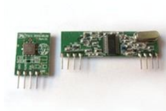
Fig. 2 Transmitter and Receiver (A434 ASK module)
