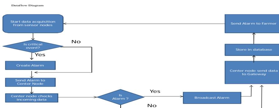
Fig2. Data Flow of Alarm System
