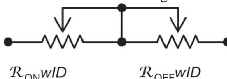
Fig. 5 Electrical Structure of the HP Memristor [3]
