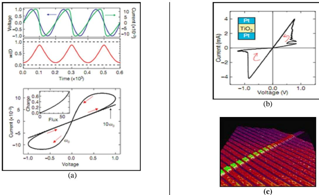
Fig. 6(a) characteristic voltage-current curve, (b) actual calculated I-V curve in TiO<sub>2</sub>, (c) AFM diagram with 17 Memristor [3] [11]
