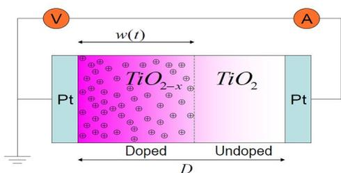
Fig. 3 Cross-section of the first HP TiO<sub>2</sub>-memristor consisting of a high conductive (doped) and a low conductive (undoped) part Placed in between two platinum electrodes. [8] Courtesy of C. Lütken.
