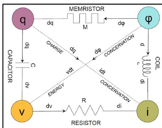
Fig. 1 Symmetry diagram showing the 6 distinct possible Realizations based on the four circuit variables. Courtesy of C.Lütken [8].
