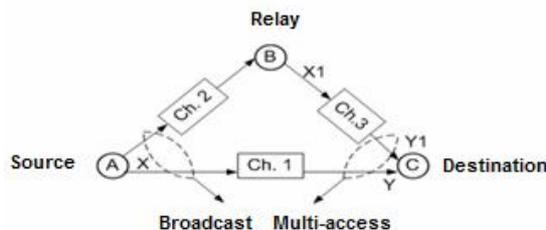
Figure 3: Relay Channel
