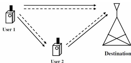
Figure 4: In Cooperative Communication each mobile is both a relay and a user
