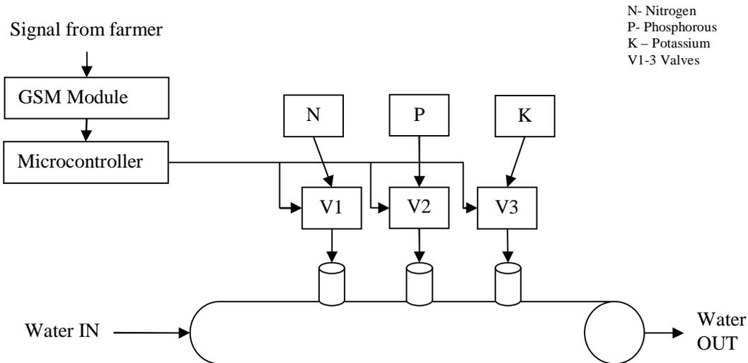
**Figure 4: Fertilization System**
