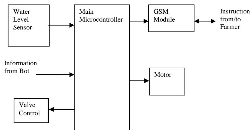
**Figure 1: Irrigation system**
