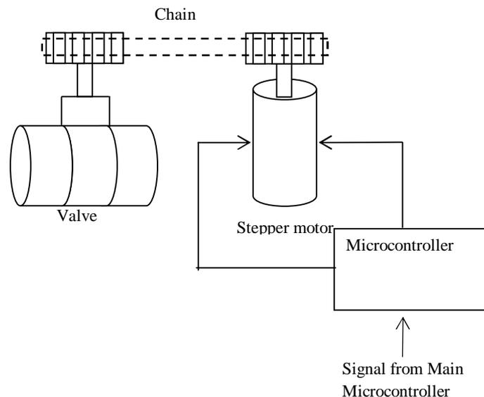
**Figure 3: Valve Control System**
