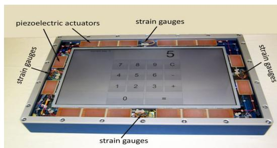
Fig.2 piezoelectric actuator with control system.
