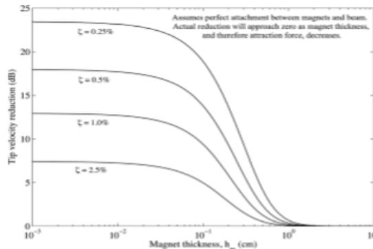
Fig.8 Tip velocity reduction using resonant shunt control for various magnet thickness & damping ratios.
