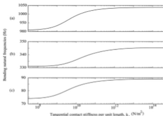
Fig.5 Illustration of the three bending natural frequencies for different contact stiffness.
