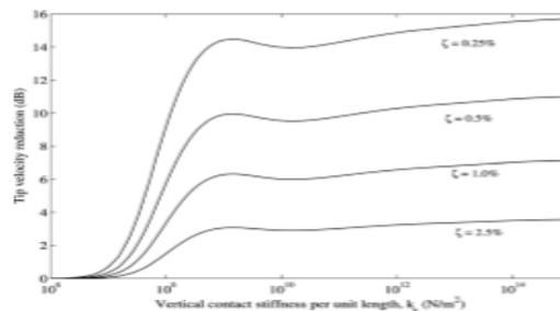
Fig.7 Tip velocity for various contact stiffnesses & damping ratios using resonant shunt control.
