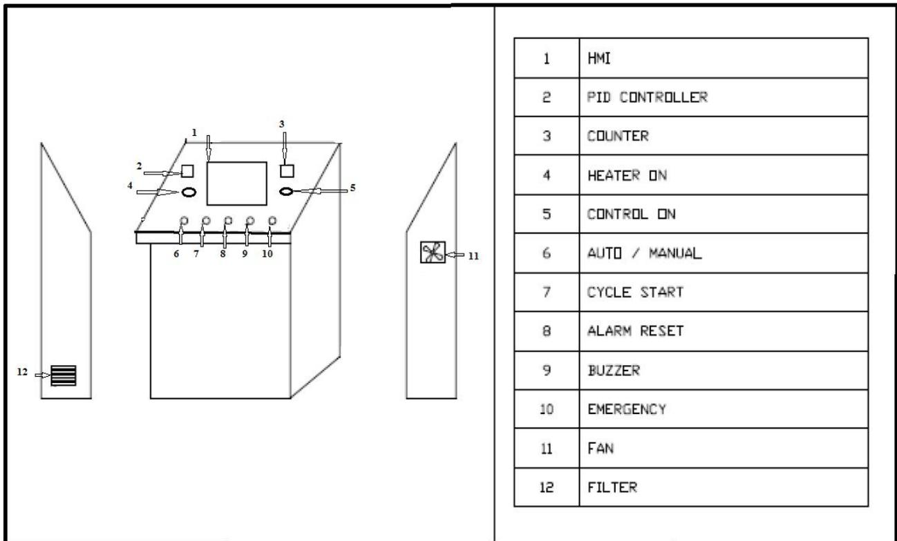
Fig.3 Block Diagram of control panel.
