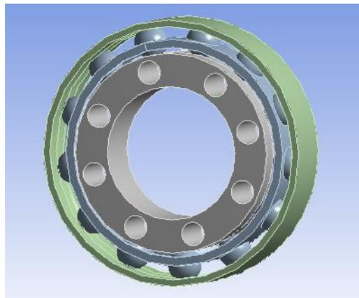
Fig. 8.1: CAD model of bearing with material removal
