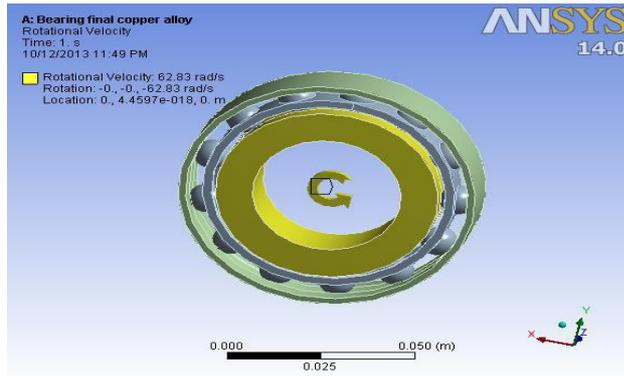
Fig. 6.2: Application of angular velocity in ANSYS
