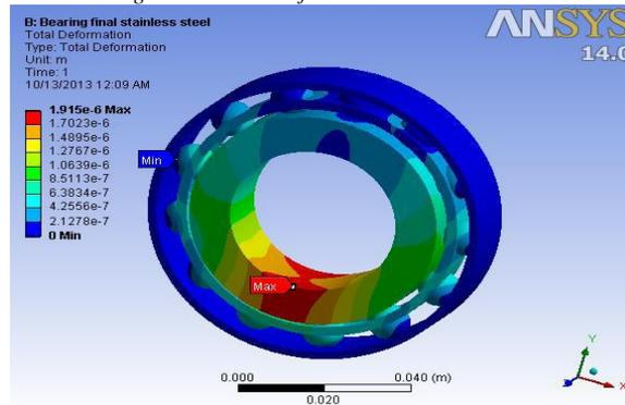
Fig. 6.4: Total Deformation
