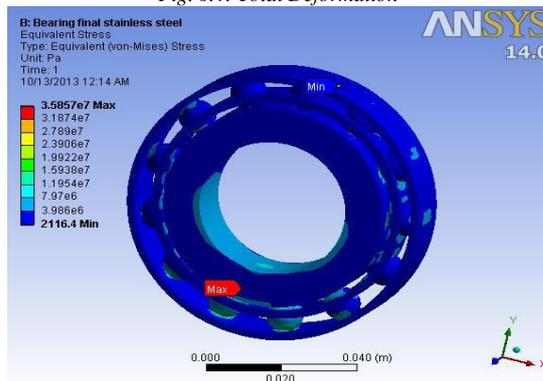
Fig. 6.5: Equivalent Stresses
