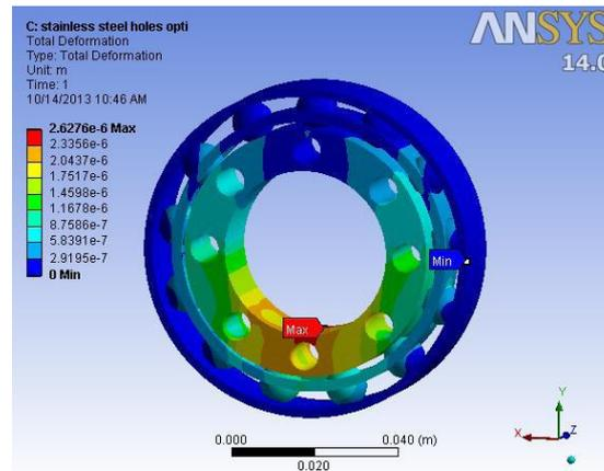
Fig. 8.3: Total deformation in the bearing
