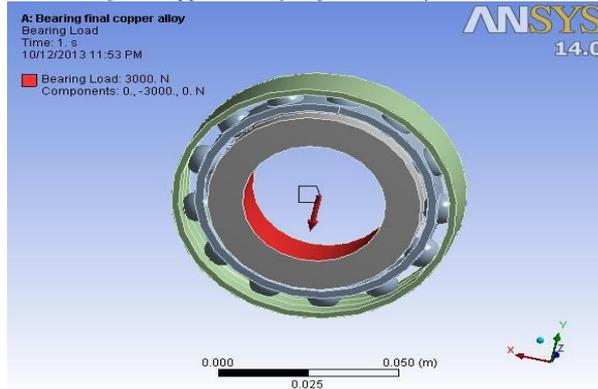
Fig. 6.3: Radial shaft load on the inner race
