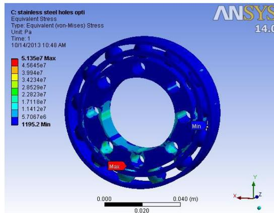
Fig. 8.2: Equivalent stresses in the bearing
