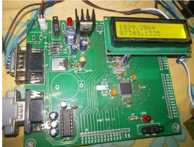
Fig.4. Coordinates Are Displayed On LCD through GPS
