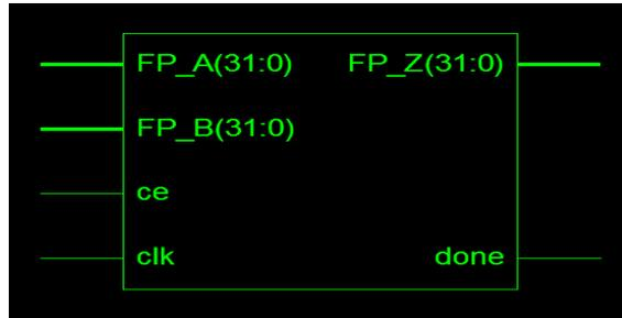
Fig. 5. Schematic representation of Multiplier
