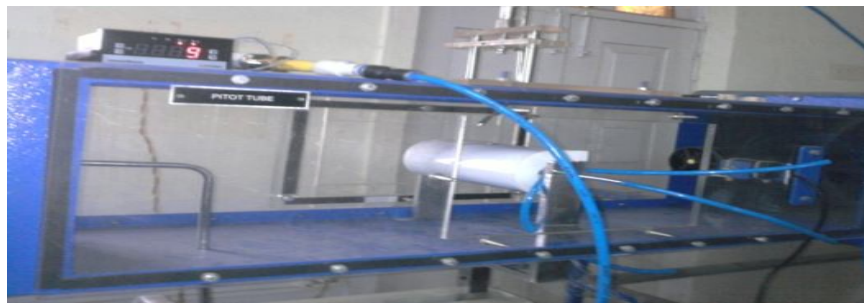
Fig.2 Fabrication of Model in wind tunnel with S-10 transmitter.
