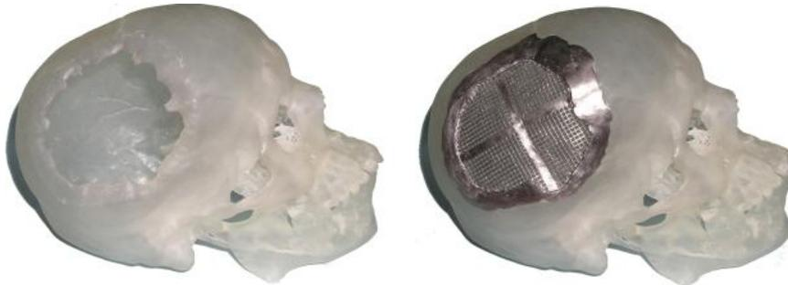
Fig. 1 Skull biomodel of an injured girl for surgical planning fabricated with SLS.
