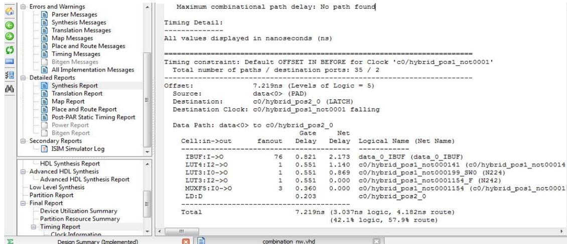
Fig. 7 Delay of HP SRAM based TCAM
