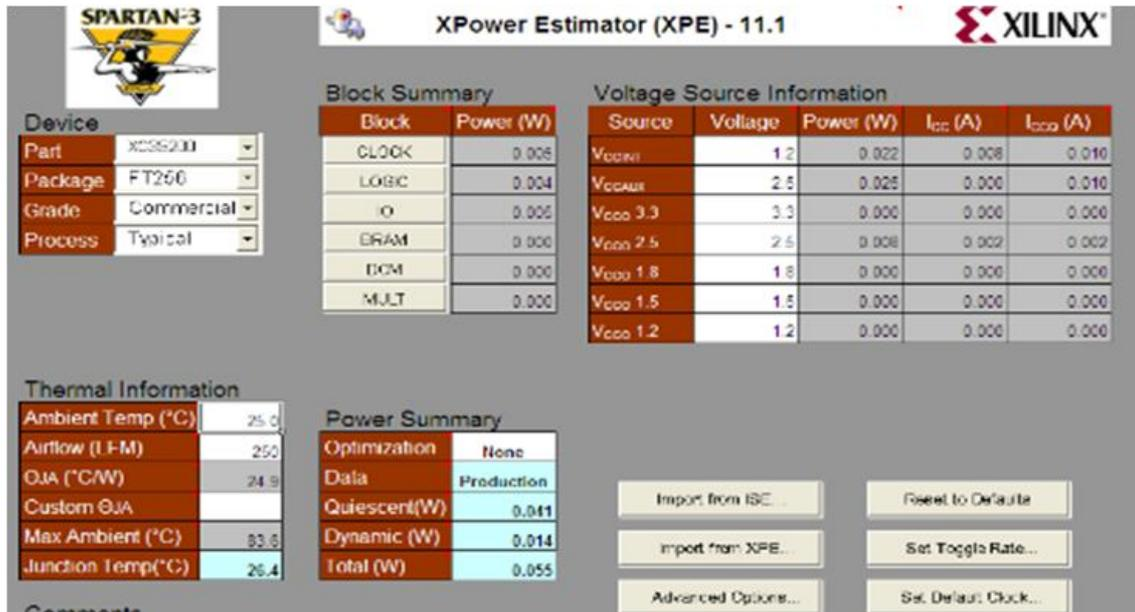
Fig. 10 Power of HP SRAM based TCAM with a Parity Bit
