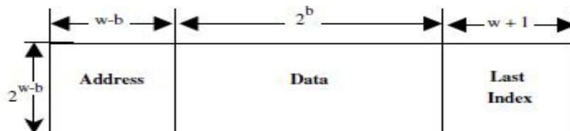
APTAG generates an address referred to APTA, which contains 1’s counter and adder. The 1’s counter counts the number of ones in the selected row of BPT and then forwards this information to adder. The adder then adds the 1’s counter output and LI of the selected row. Fig. 4 shows the conceptual view of APT, where  $K$  bits represent the number of bits in each row.
