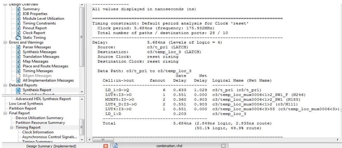
Fig. 8 Delay of HP SRAM based TCAM with a Parity Bit
