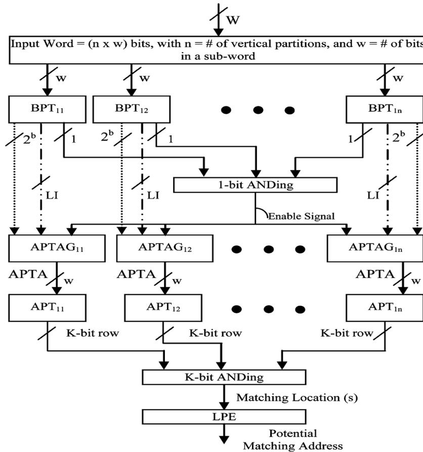
Fig. 2 Architecture of a layer of HP SRAM based TCAM
