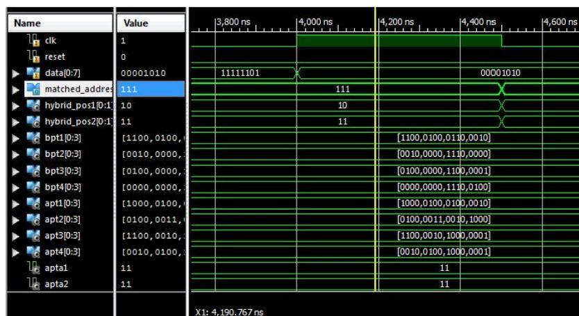
Fig. 6 Simulated Waveform of HP SRAM based TCAM with a Parity Bit
