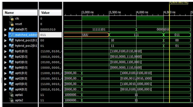
Fig. 5 Simulated Waveform of HP SRAM based TCAM
