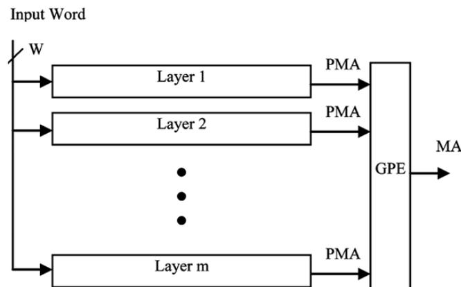
Fig. 1 Memory Architecture of HP SRAM based TCAM
