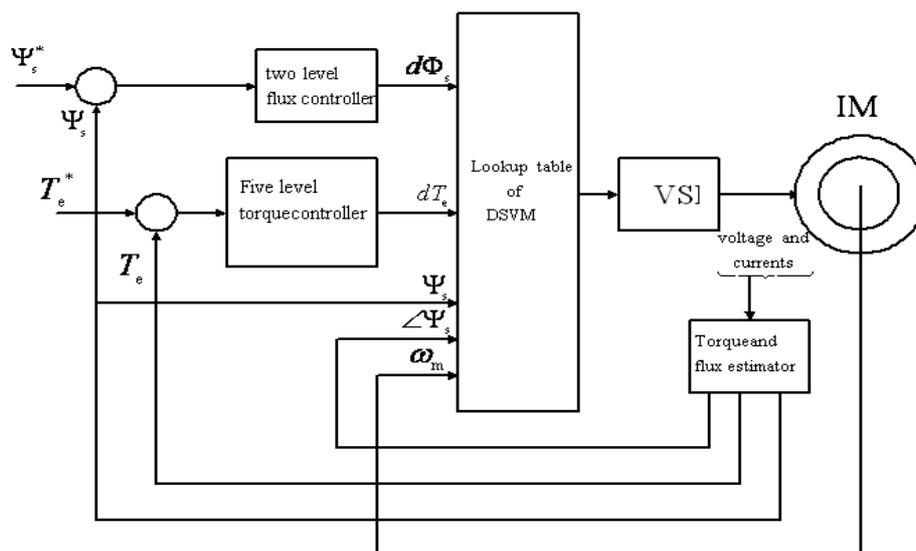
**Figure 3 Block diagram of Discrete SVM-DTC**
