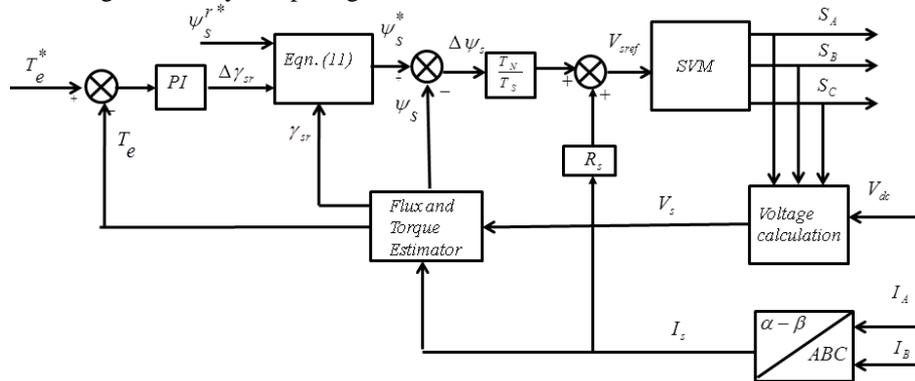
Figure 7 SVM DTC with torque control
