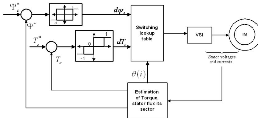
**Figure 2** Block diagram of classical DTC scheme
