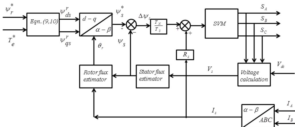
**Figure 6 Block diagram of SVM-DTC with flux control**
