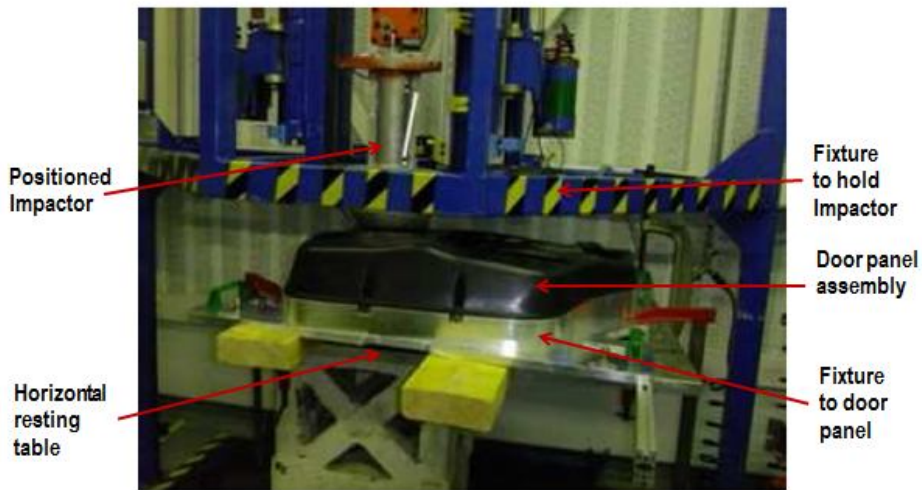
Fig.8 Physical testing setup
