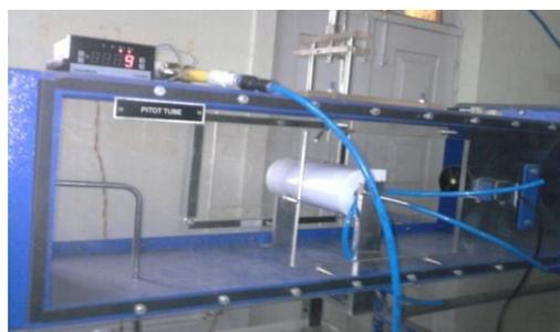
Fig. 5: Fabrication of Model in wind tunnel with S-10 transmitter.
