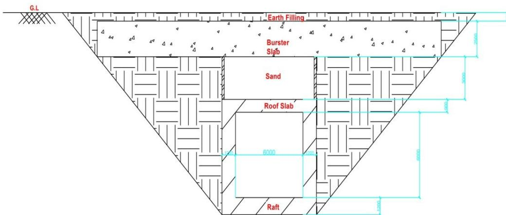
**SECTIONAL PLAN OF AN UNDERGROUND STRUCTURE**
