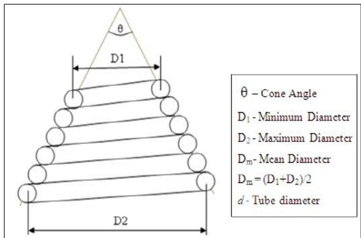
Fig.2 A Geometry of conical coil
