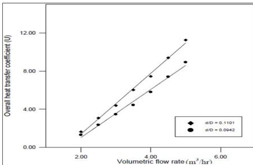
Fig.4: The effect of the curvature ratio of coil on the overall heat transfer coefficient
