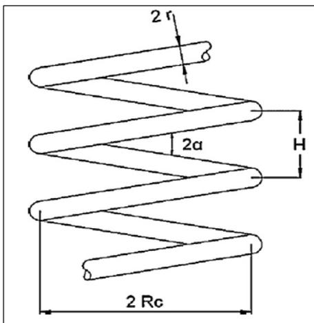
Fig. 1 A Geometry of helical coil
