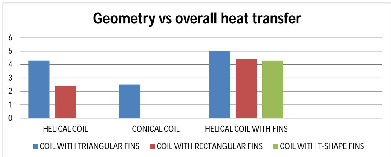
Fig.5 Geometry vs overall heat transfer
