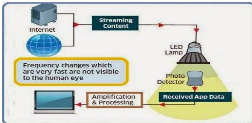
Figure 2 : Li-Fi System Block Diagram
