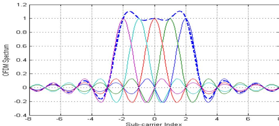
Figure 9: OFDM modulation subcarrier
