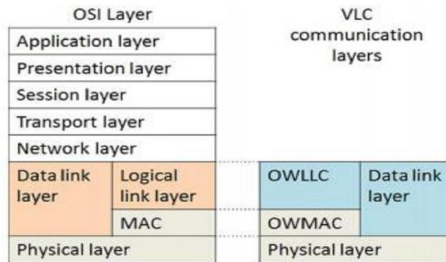
Figure10:OSI reference model for VLC communication
