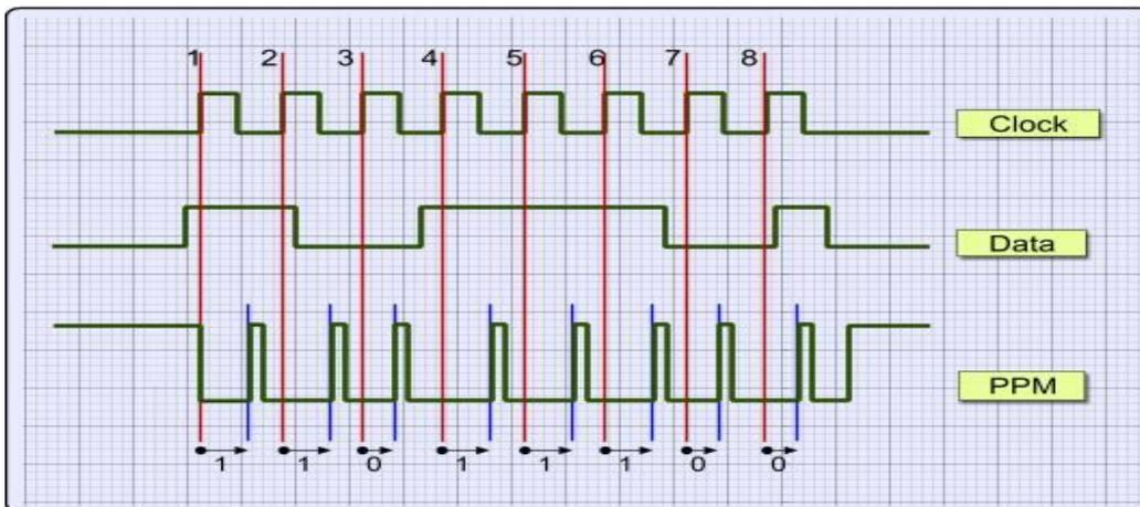
Figure 8: Shape of pulse position modulation
