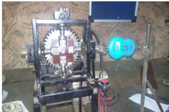
Fig. 2 Experimental Setup of Biaxial tensile testing machine
