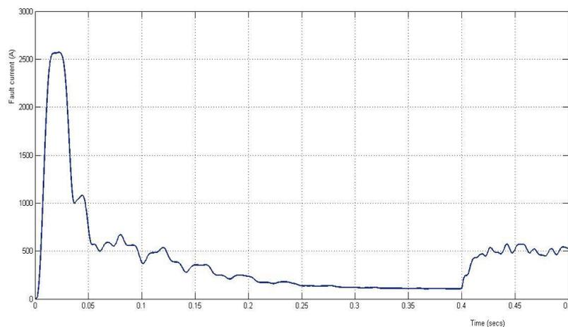
Fig.14. RMS value of fault current for Fault 2 with SFCL at Location 1 and Location 4
