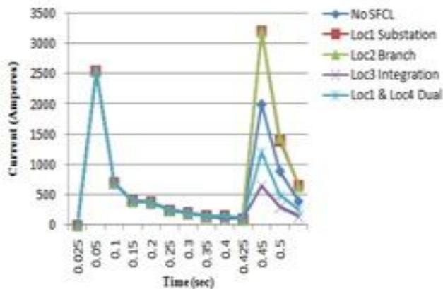
Fig.9. Comparison of wind farm fault currents for four SFCL locations in case of fault in distribution grid (Fault 1)
