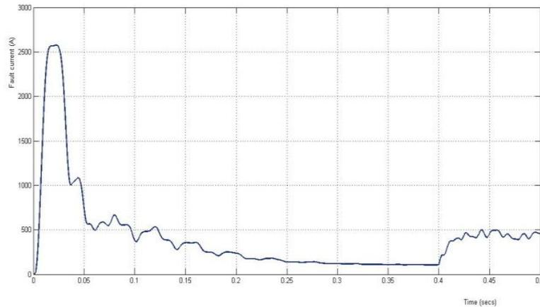
Fig.13. RMS value of fault current for Fault 2 with SFCL at Location 3
