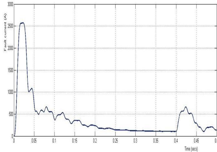
Fig.7. RMS value of fault current for Fault 1 with SFCL at Location 3
