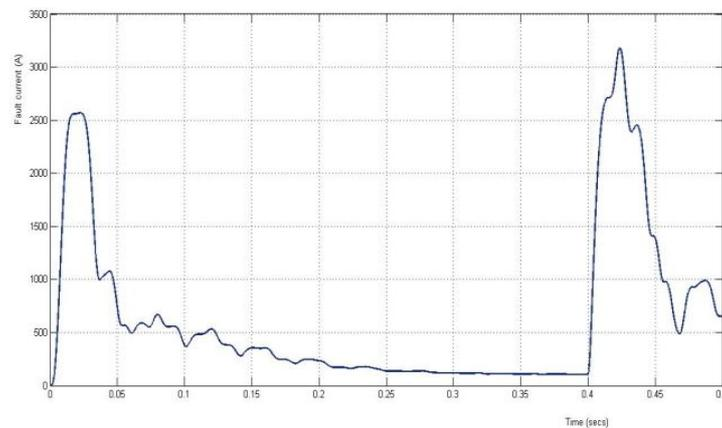
Fig.6. RMS value of fault current for Fault 1 with SFCL at Location 2
