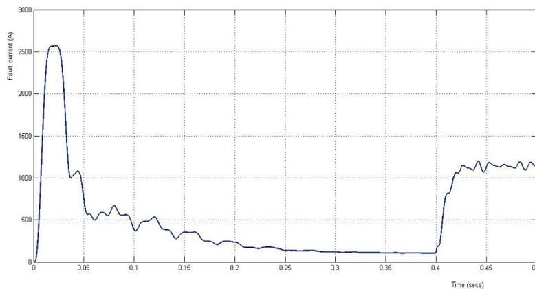
Fig.11. RMS value of fault current for Fault 2 with SFCL at Location 1
