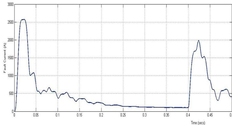
Fig.4. RMS value of fault current for Fault 1 without SFCL
