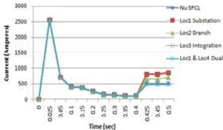
Fig.15. Comparison of wind farm fault currents for four SFCL locations in case of fault in customer grid (Fault 2)
