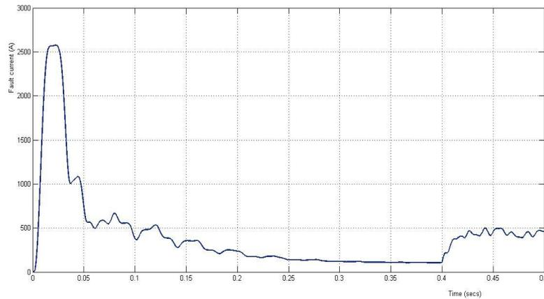
Fig.10. RMS value of fault current for Fault 2 without SFCL
