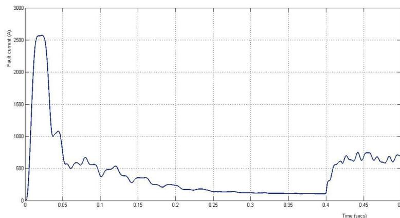
Fig.12. RMS value of fault current for Fault 2 with SFCL at Location 2
