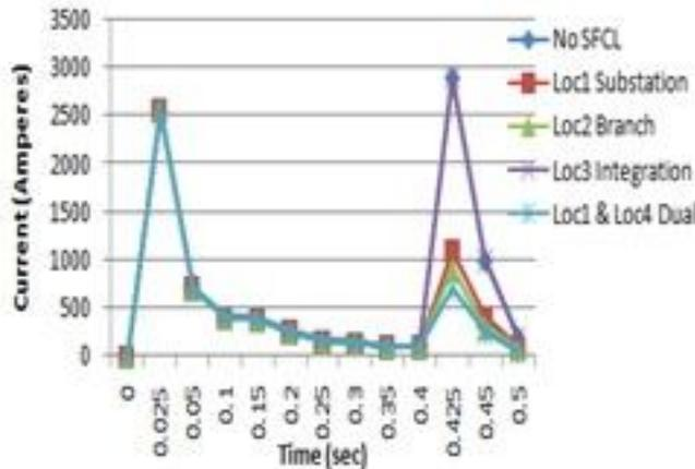
Fig.16. Comparison of wind farm fault currents for four SFCL locations in case of fault in transmission line (Fault 3)
