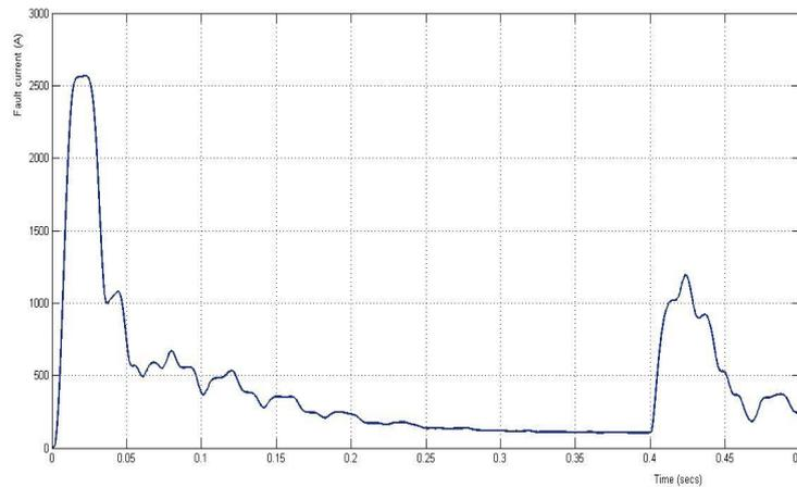
Fig.8. RMS value of fault current for Fault 1 with SFCL at Location 1 and Location 4
