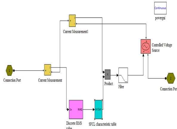
Fig.2. Single phase Resistive SFCL Simulink model
