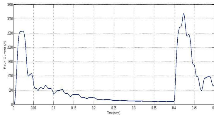
Fig.5. RMS value of fault current for Fault 1 with SFCL at Location 1
