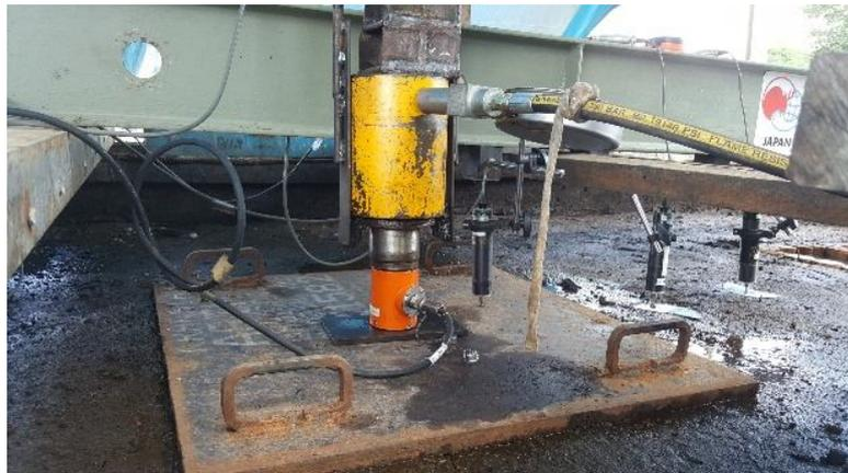
Fig. 4 Axial loading test of soil
