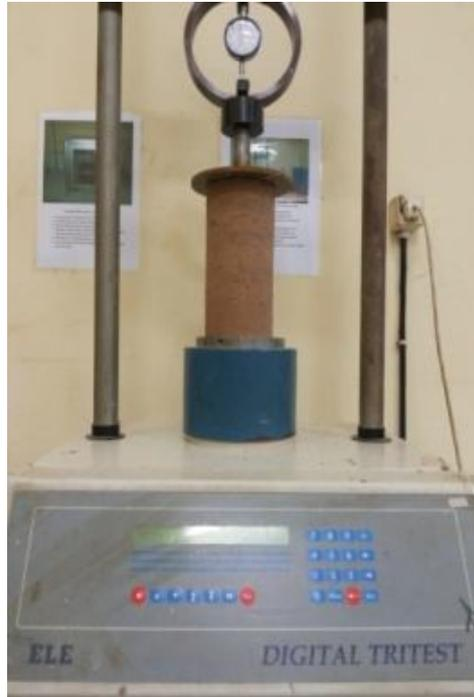
Fig. 4 Unconfined compression test
