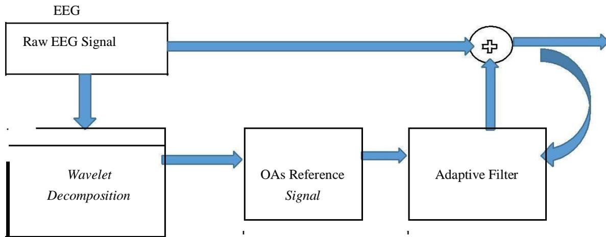
Figure 1 OA removal model combining DWT and ANC
