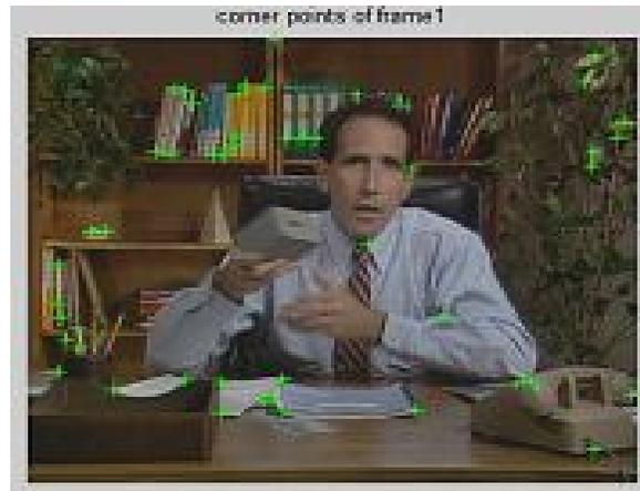
Figure3: Corner points detected of frame
