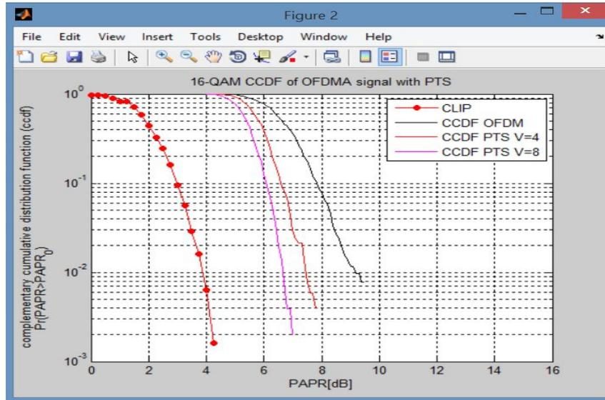
Fig 2: Figure shows the complementary cumulative distribution function (ccdf) versus peak to average power the clipping and filtering, partial transmit sequence (v=4), partial transmit sequence (v=8) and orthogonal frequency division multiplexing
