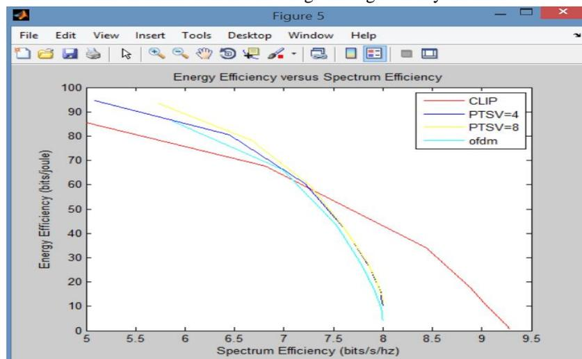
Fig 3: Figure shows the energy efficiency versus spectrum efficiency of the clipping and filtering, partial transmit sequence(v=4),partial transmit sequence(v=8) and orthogonal frequency division multiplexing
