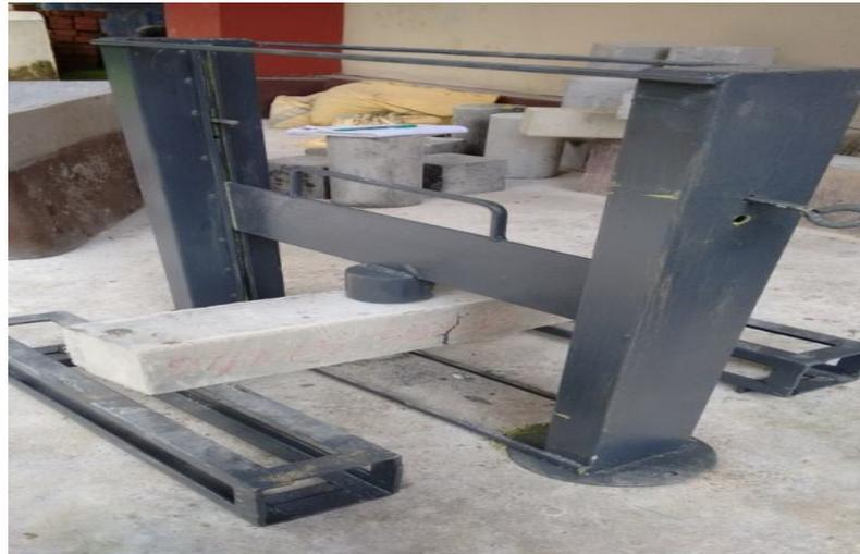
Fig. 1 Impact test rig with specimen
