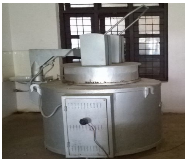
Fig. 1 Electrically Heated Air Circulating Furnace
