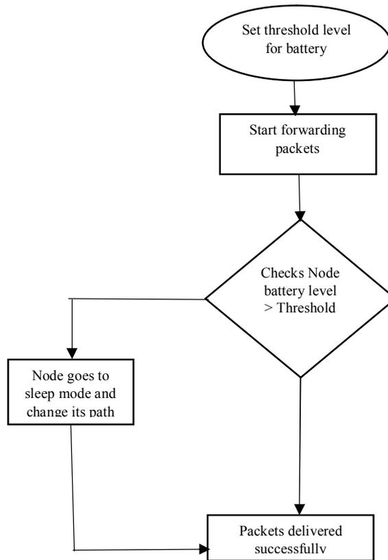
Figure 4.3 : DPS flow diagram
