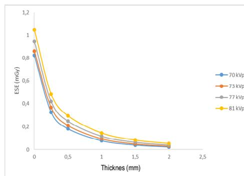
Figure 5. ESE value with AlZnSi thickness variation
