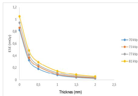
Figure 6. ESE value with Zn thickness variation
