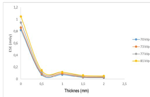
Figure 4. ESE value with Cu thickness variation
