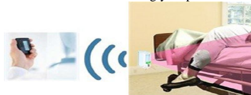
Wireless signaling between PIR motion sensor and the caregiver pager
