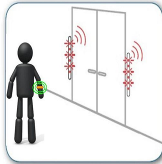
An example of the anti-wandering wristband based door alarm system
