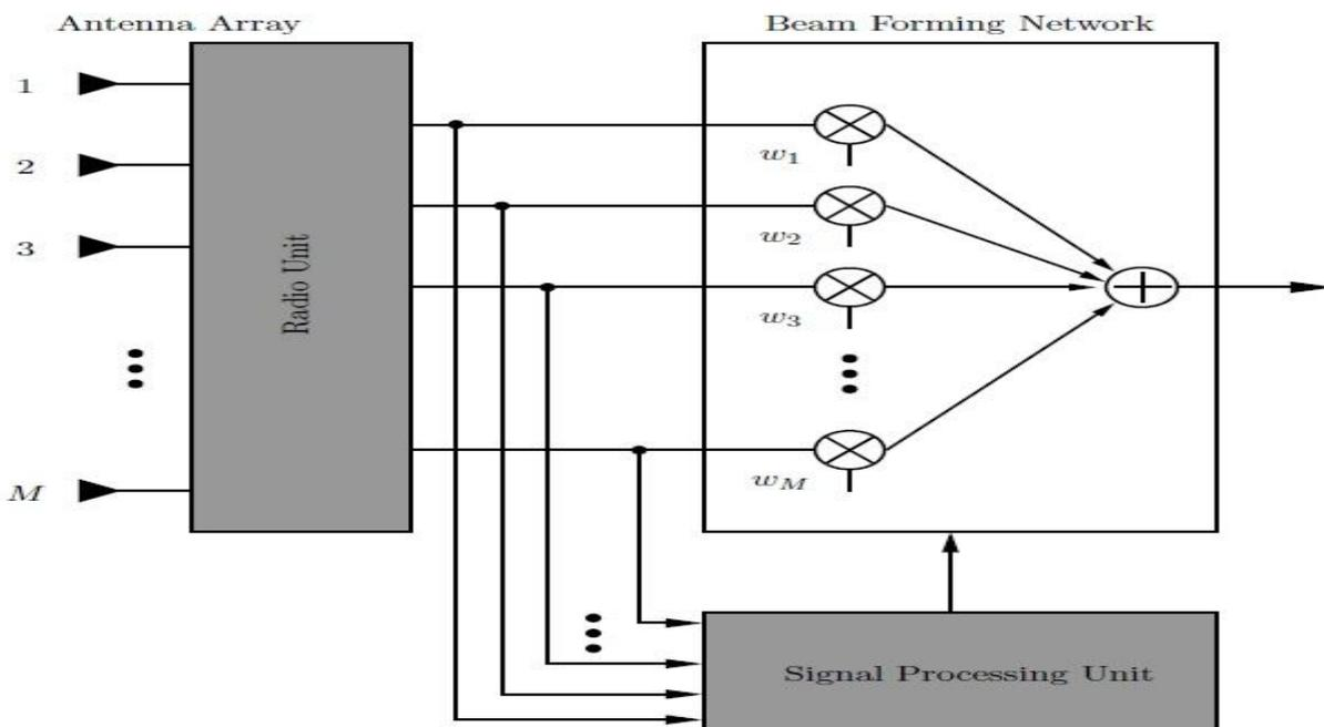
Fig 2- Smart antenna Receiver
