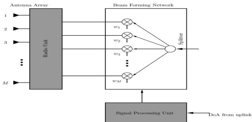
Fig 3- Smart antenna transmitter
