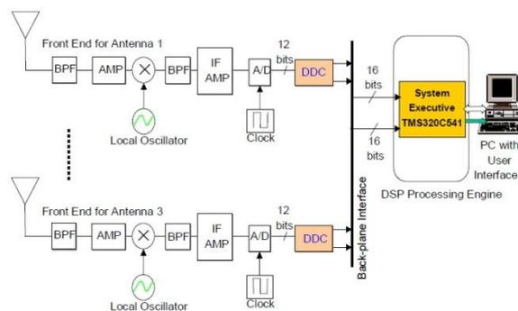
Fig 4 – Block diagram of Adaptive Array System
