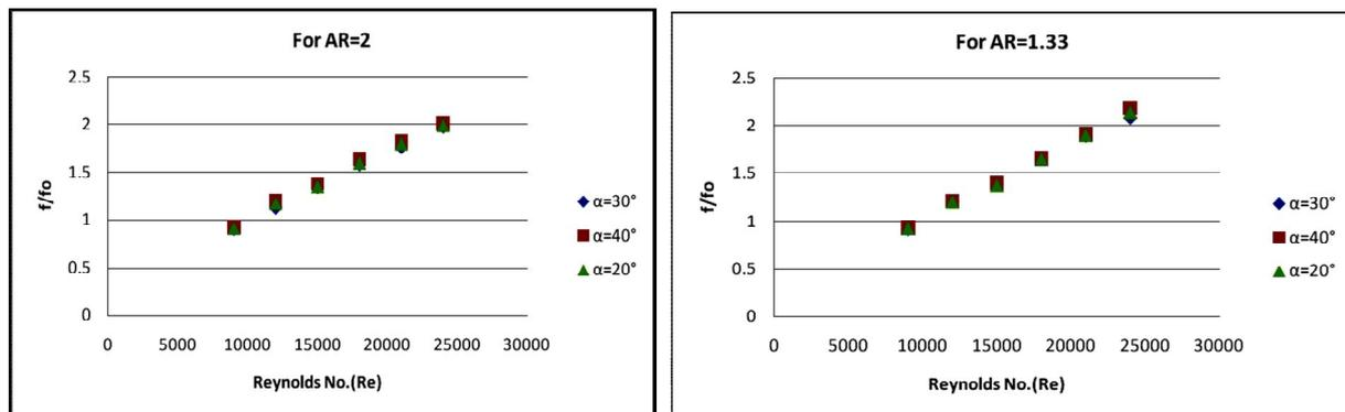
Fig. 13: Variation of Friction factor as function of Re for AR=1.33 and AR= 1.33
