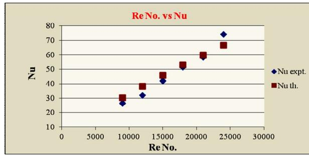
Fig.1: Nusselt Number Vs Reynolds Number for flat plate
