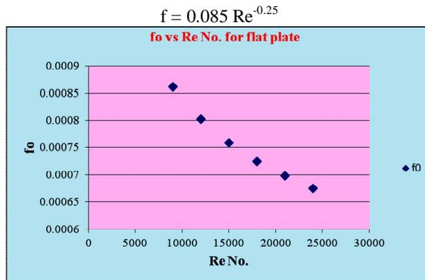
Fig.2: Friction factor vs Re for flat plate
