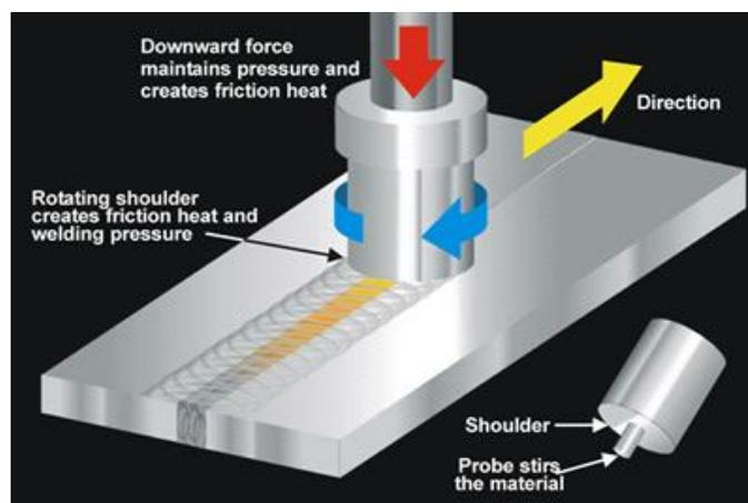
Figure: 1 Schematic diagram of FSW
