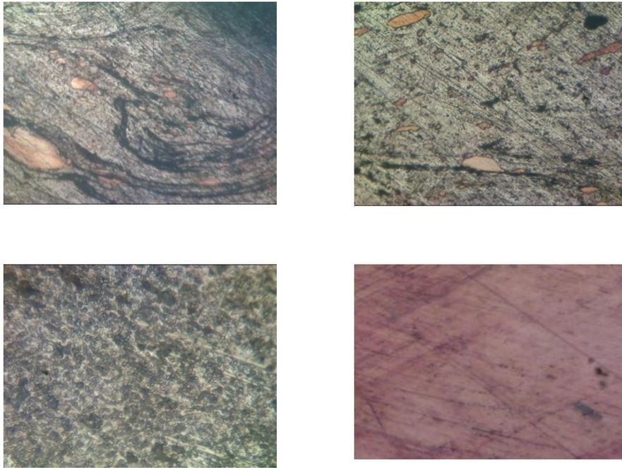
Figure: 2 Microstructure of NZ, TMAZ and HZ
