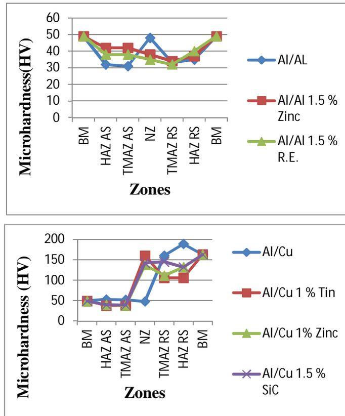
Figure:3 Microhardness values of Al/Al and Al/Cu
