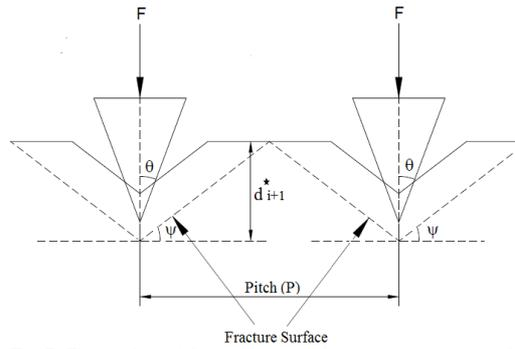
Fig 7: Physical model of interaction between adjacent teeth
