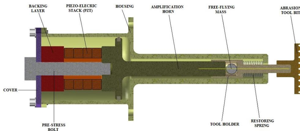
Fig 1: Schematic of Ultrasonic Percussive Rock Abrader (UPRA)
