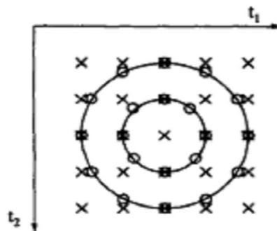
Fig. 1. Formation of rotation-invariant variables, where "x" denotes a pixel (grid point) And "O" denotes a resample point
