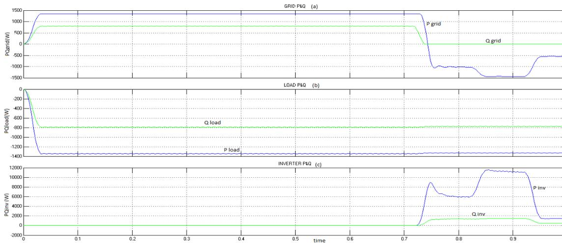
Fig. 4. Simulation results: (a) PQ-Grid, (b) PQ-Load, (c) PQ-Inverter.
