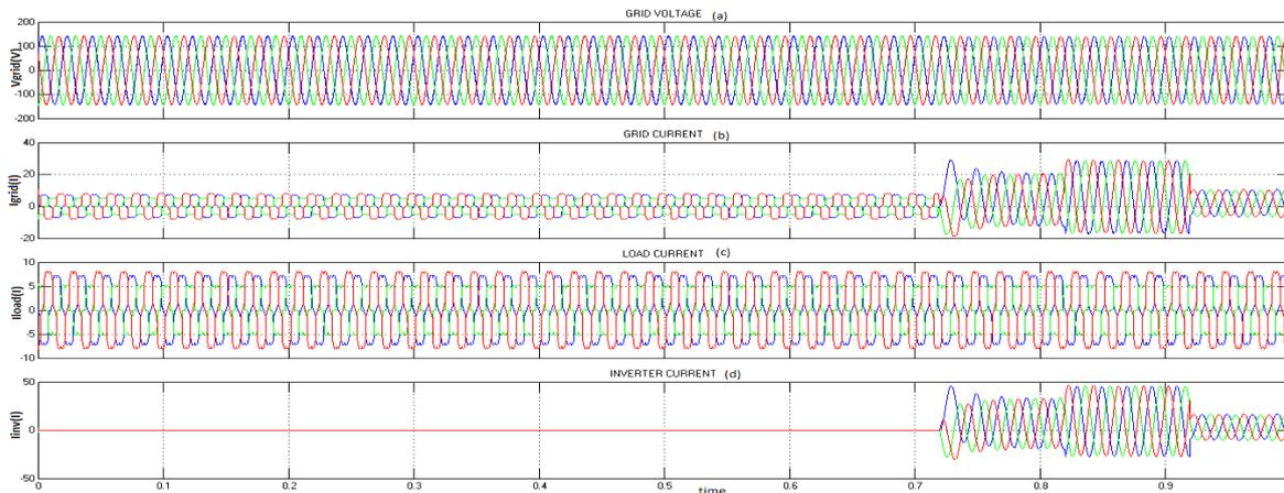
Fig. 3. Simulation results: (a) Grid voltages, (b) Grid Currents (c) Unbalanced load currents, (d) Inverter Currents.
