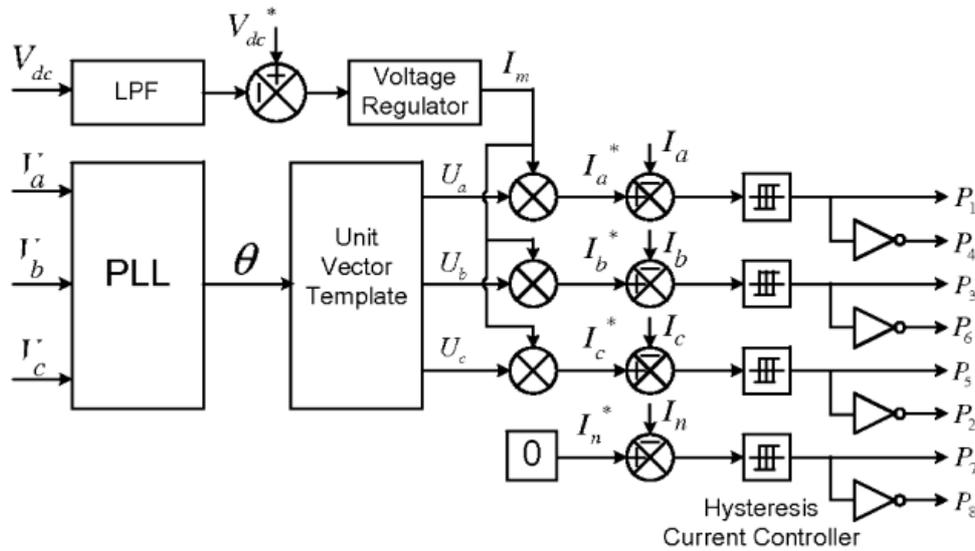
Fig. 2. Block diagram representation of grid-interfacing inverter control.
