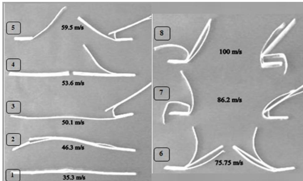
Fig. 5 Photograph showing the Sandwich beams impacted at different projectile velocity. The number written below at each beam is the impact velocity of the projectile.
