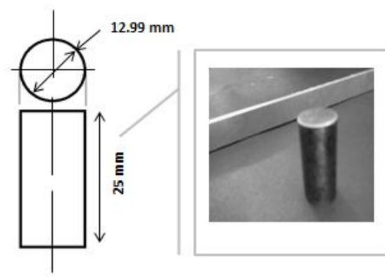
Fig. 2 Geometric layout and camera view of the blunt cylindrical projectile
