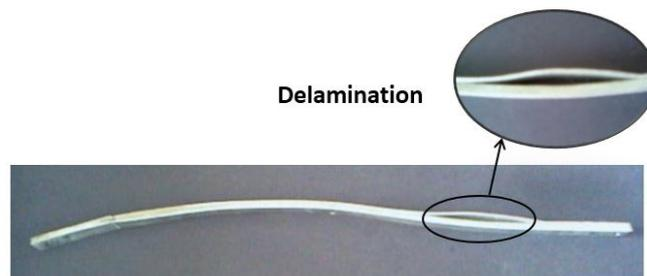
Fig. 10 Showing Delaminated area after impact
