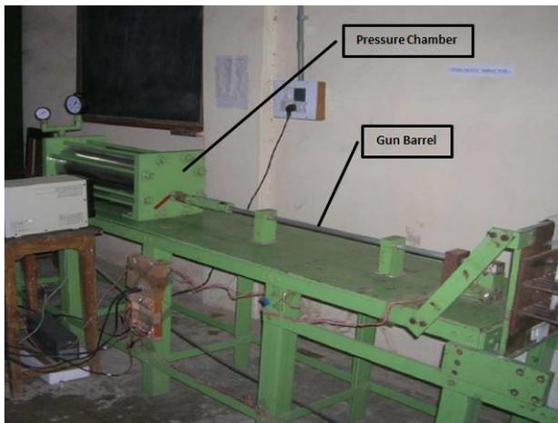
Fig. 3 Pneumatic Gun Apparatus at Aligarh (Front view)
