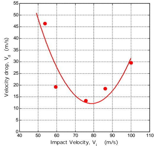
Fig. 9 Impact velocity ( $V_i$ ) versus Velocity drop ( $V_d$ )
