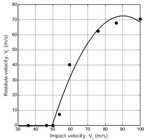
Fig. 7 Impact velocity ( $V_i$ ) versus Residual Velocity ( $V_r$ )
