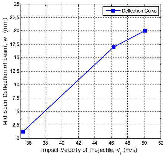
Fig. 6 Mid span deflection ( $w$ ) versus impact velocity, ( $V_i$ )
