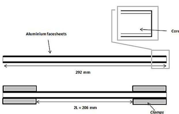
Fig. 1 Line diagram of the clamped sandwich beam.
