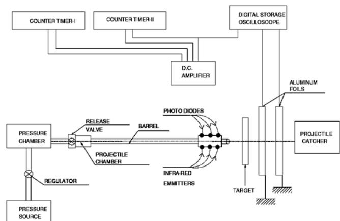
Fig. 4 Schematic of experimental set up
