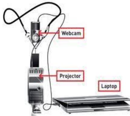
Figure-2:(a) and (b) shows hardware components: Camera/Webcam, Projector and Laptop of Sixth Sense Technology
