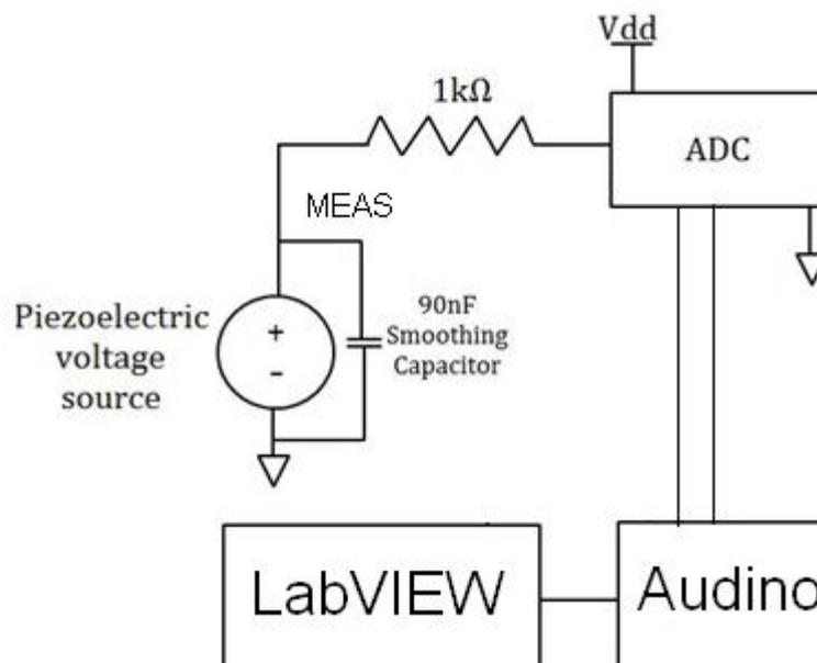
Fig3. Block Diagram- Diet Pattern analyser
