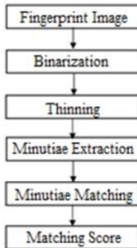
Fig 2. Minutiae based fingerprint recognition method.
